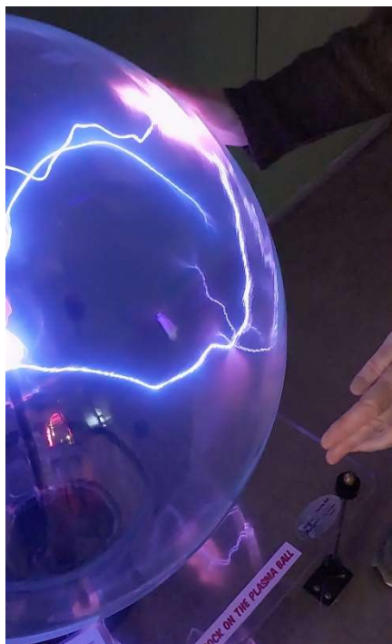
Figure 4. Plasma Ball. The arc goes from the center to the glass at the location of the object that touches the glass.
