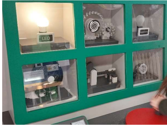
Figure 6. Turn the red crank to make one to six items work. The more items with the circuit selected the more difficult to turn the crank.
