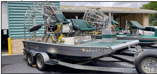
Figure 1. Picture of Fan boat. Note the big white spray tank between the front and rear seats.
