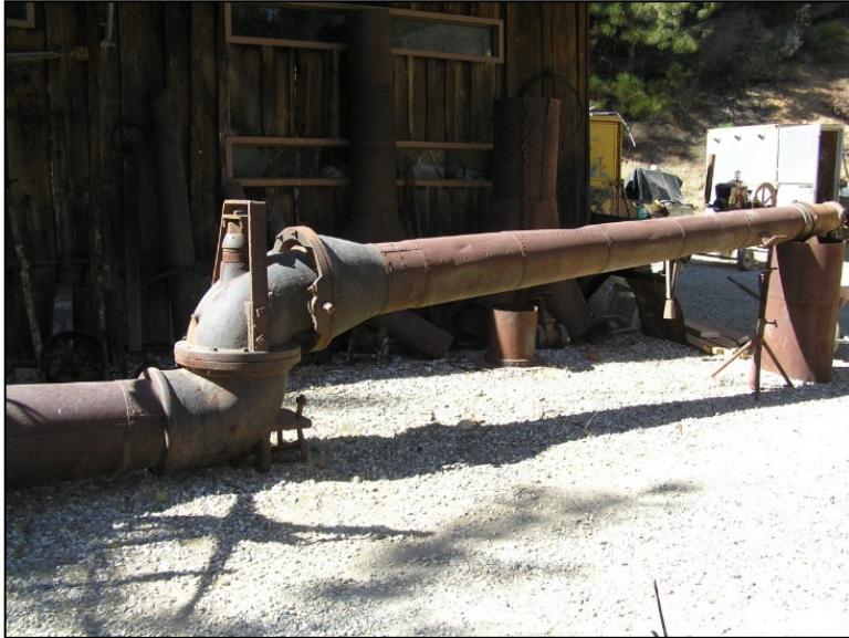
Figure 4: Large monitor on display at Waukeshaw Drift Mine, Relief Hill, CA. Photo by W.E. Motzer, October 2009.
