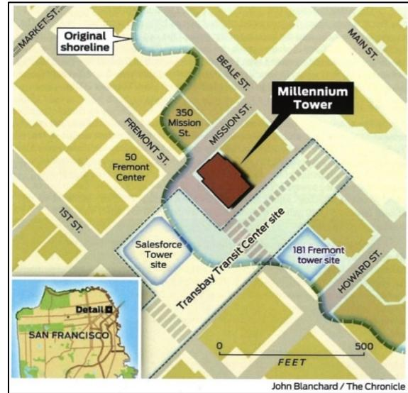
**Figure 5:** Millennium Tower (301 Mission Street) location in relation to original shoreline and fill area. Building pilings were anchored 80 feet (~24 m) below ground surface (bsg) into packed sand with bedrock at ~250 feet (~76 m) bsg. Subsidence rate was ~40 mm per year for a total of 46 cm by 2018 resulting in a leaning of 36 cm. Dewatering during construction of the adjacent Transbay Center site may have contributed to the subsidence. Source: Sullivan (2017).
